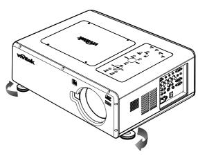
**2.** To lower the level of the projector, lift the projector and twist the adjusters counter clockwise.
